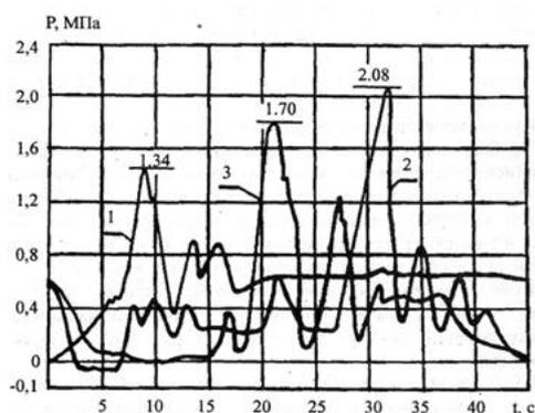
**Fig. 3.** Oscillograms of pressure changes in a 600 mm diameter main pipeline when 20P-11-type pumps are connected following the “pump in pump” scheme sequential circuit:
