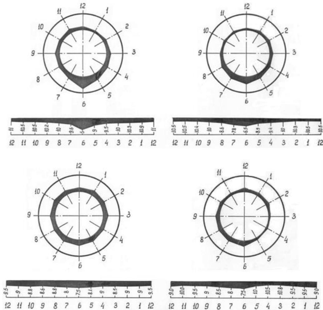
**Fig. 1.** Distribution diagrams of hydroabrasive wear of hydrotransport system main pressure pipeline ( $D=426$  mm) straight portion with slurry moving in them in various modes (with various parameters)
