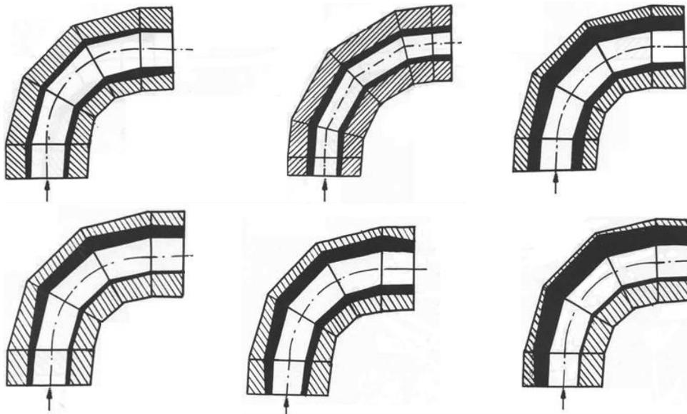
**Fig. 2.** Distribution diagrams of hydro-abrasive wear of hydro-transport system main pressure pipeline (D=426 mm) curvy portion (of turns) with slurry moving in them in various modes (with various parameters)
